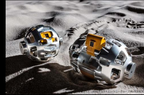
SORA-Q (LEV-2), the world's smallest and lightest transformable lunar exploration robot, developed by JAXA, TAKARATOMY, SONY and Doshisha Univ. ©JAXA
